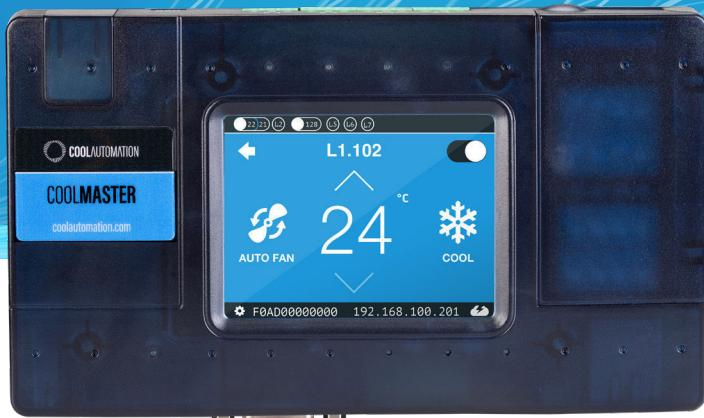
CoolMaster allows automation integrators, facilities managers, service providers and HVAC professionals the ability to control, monitor, service, and manage any VRF, by enabling a bi-directional universal communication channel between the VRF HVAC and the automation systems. CoolMaster is a Plug & Play device - simply unbox it and connect it to your VRF HVAC System.
